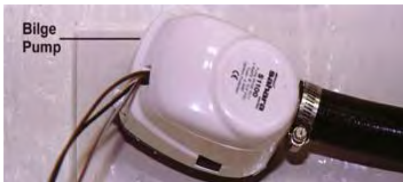
Bilge Pump is Mounted to ABS Plastic
