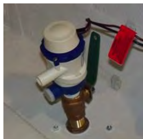
Livewell Pump Assembly in the “OPEN” Position
