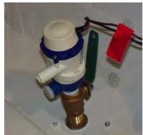
Livewell Pump Assembly in the “OPEN” Position
