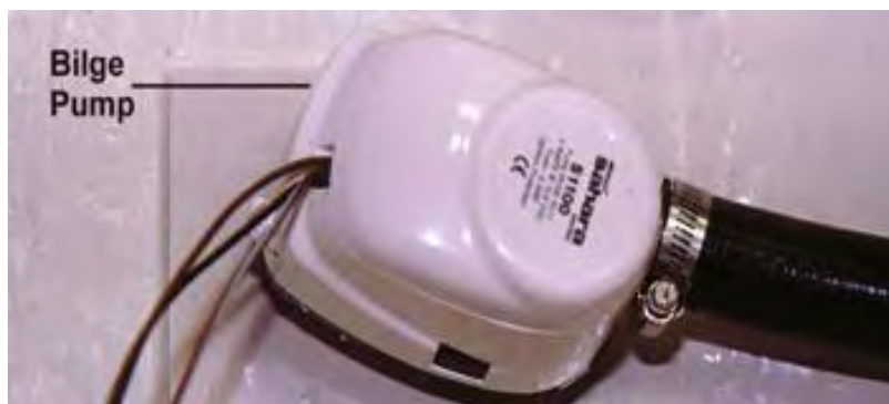
Bilge Pump is Mounted to ABS Plastic
