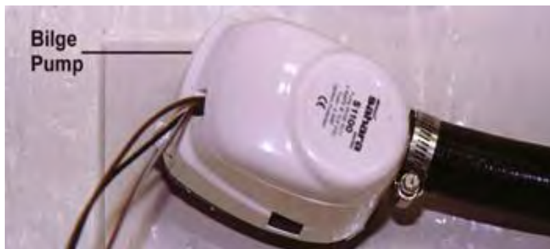
Bilge Pump is Mounted to ABS Plastic
